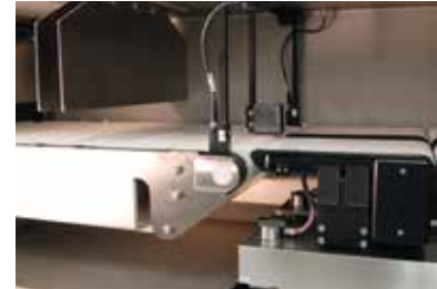
Comprehensive product inspection: X-Ray and weighing in combination
